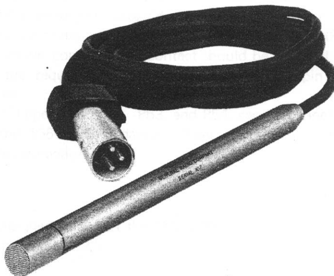
Figure 4-1. Type 1560-P42 Preamplifier with microphone attached.
